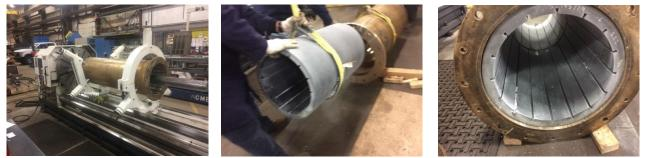
These photos show the refurbishment of the bronze carriers underway in a machine shop in Dartmouth, NS and fitting of the Thordon XL bearings.
