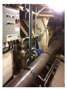
These photos show the original shaft packing gland and the new SeaThigor inboard shaft seal during installation. The new Thordon WQP is shown during commissioning fitted very snuggly into the starboard shaft tunnel The main shaft is in the foreground.
