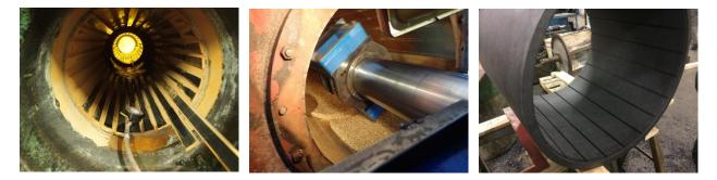
The outcome was a series of contracts between CCG and Avalon Marine to engineer, assess, submit and obtain the Class approvals as well the design the bearing upgrades and shipboard equipment integration. Thordon and Avalon supplied three full shaft line sets of Full form Thordon XL bearings and three custom water quality packages to continuously condition the bearing lubrication water. This contract was unique as it was the first time WQPs
