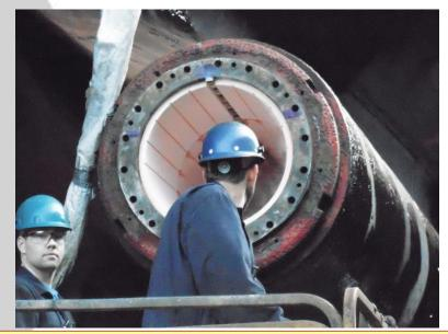
CCGS Des Groseilliers Type 1200 – Fitted with COMPAC bearings 2012.
