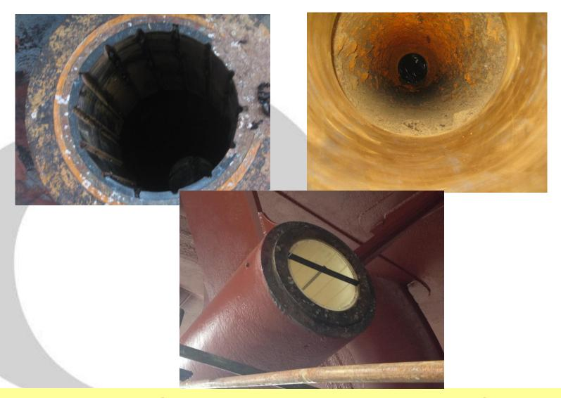
MV Venture Sea – supply ship replaced Cutlass bearings with Thordon SXL full form bushings.
