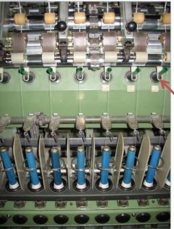
Example of "Ring Spinning Frame" used to spin fibres to make yarn
